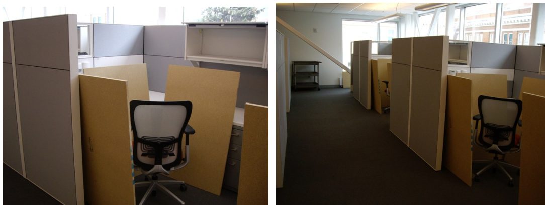
Figure B-1 Contaminant source introduced into the test room by using particleboards
